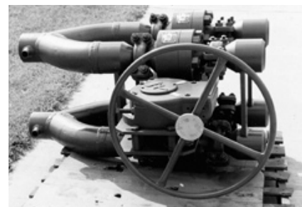
Unique custom-built valve configuration consists of four, 2-inch ASME 1500 Class valves with operating conditions of 300°F at 2600 psi (149°C at 179 bar). The valves were linked for a specific sequence in order to synchronize open/close of bypass lines.
