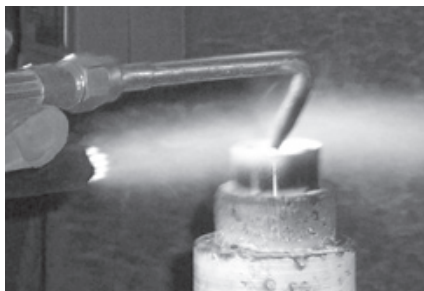
Using the latest technology, this seat is receiving a spray and fused coating. MOGAS coatings are specially chosen to handle the operating conditions of each application.
